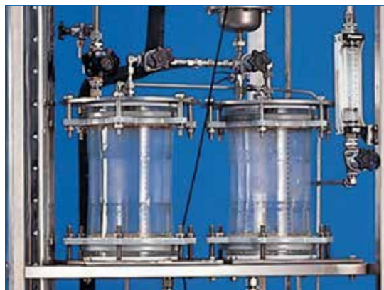
Receiver vessels being cleaned using integral CIP facility.
