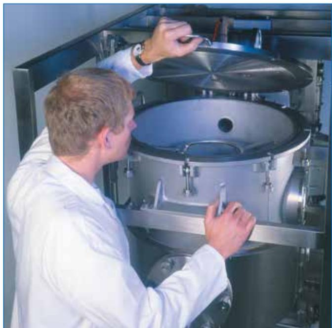
Inspecting the interior of the extractor vessel
